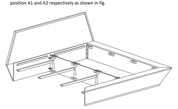
Now place Part-C(Battens) at bottom U-block as shown in Fig.
