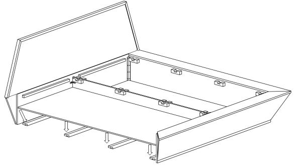
Now place Part-E(Bottom panel) into last assembled part as shown in fig.
