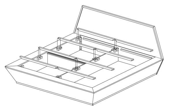
Now place Part-C (Battens) at bottom U-block as shown in Fig.
