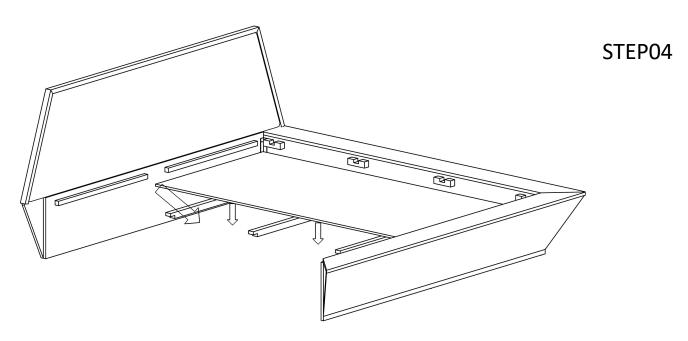
Now place Part-E(Bottom panel) into last assembled part as shown in fig.
