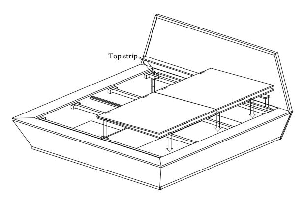
Now place Part-I (Top strip) and Part-H(Top panel) at last assembled as shown in Fig.
