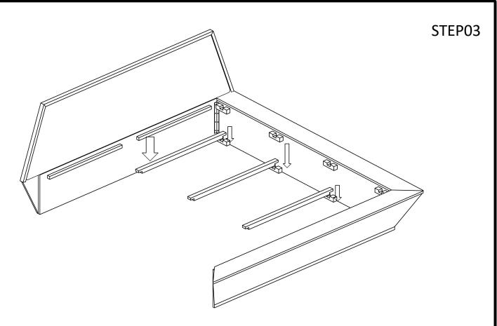
Now place Part-C (Battens) at bottom U-block as shown in Fig.
